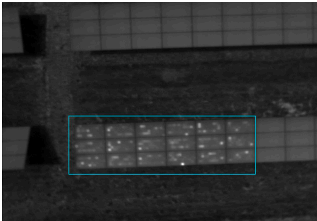
Figure 6: Example of a Reverse Polarity Anomaly Detected by Raptor Maps
